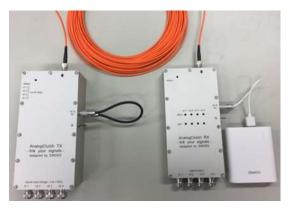
MOE-ACTx/Rx enable to convert the Analog Voltage to Optical signal for the EMC inspection and could transfer the electric signal of EUT (Equipment under test) in chamber room by using Optical-Fiber to the outside measurement equipment. The radiation noise of this analog clutch is suppressed as much as possible not to influence EMC inspection.
